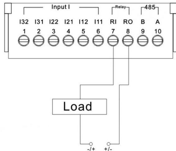
Input&output Wiring diagram
