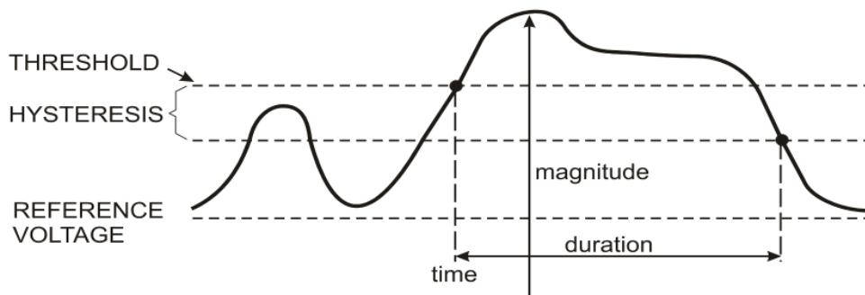
The voltage drops during the dip. In a three-phase system, when the voltage of one or more phases drops to the dip threshold, the dip begins; When the voltage of all phases is equal to or greater than the dip threshold plus Hysteresis, the dip stops. The trigger conditions of sudden drop are threshold and Hysteresis. Sudden drop is characterized by duration, amplitude and occurrence time.
