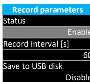
"Status" is used to set whether data storage is enabled. When it is disabled, data will not be stored in internal memory.
