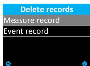
"Measured value record" is used to delete records of basic data, voltage harmonic data and current harmonic data.
