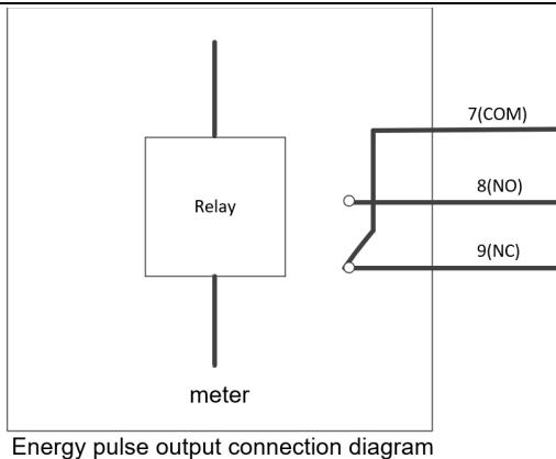
Energy pulse output connection diagram
