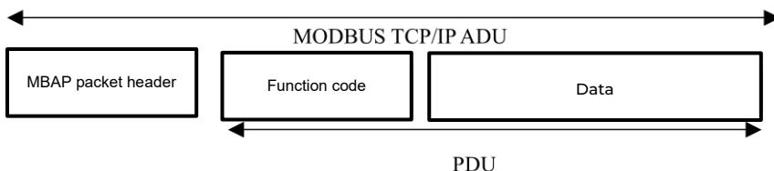
MBAP mesdipe header(MBAP、Modbus Application Protocol、Modbus application Protocol) is divided into 4 fields with 7 bytes in total, as shown in the figure below:
