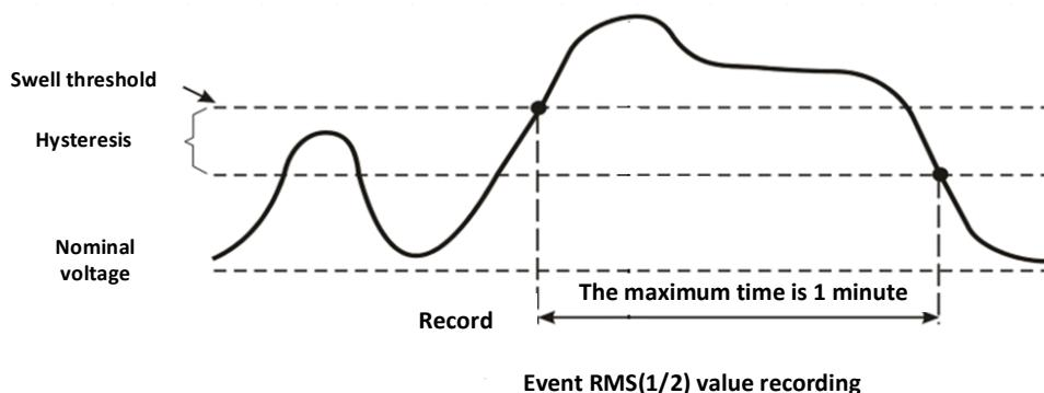
The waveform recording adopts a fixed sampling rate of 8kHz, and the recording is divided into four parts: before the beginning of event, after the beginning of event, before the ending of event, after the ending of event.
