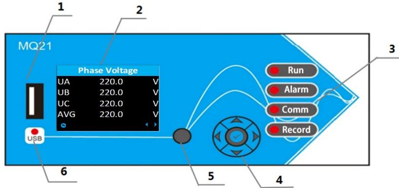
The analyzer adopts OLED display, 1 independent push button and 1 five way push button, as shown in the figure below:
