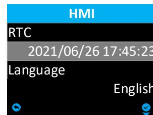
The selected content can be switched through key and key , press key to enter the setting interface, and press key to exit the current interface.
