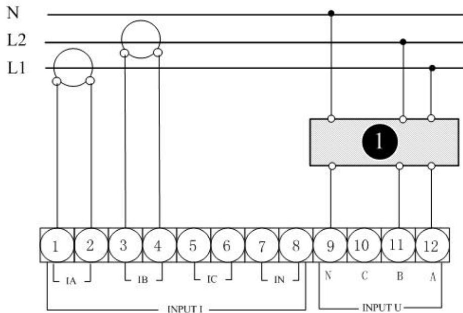
ModBus communication &output Wiring diagram
